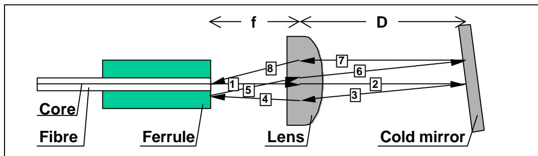
Figure 4: Double pass delay line
