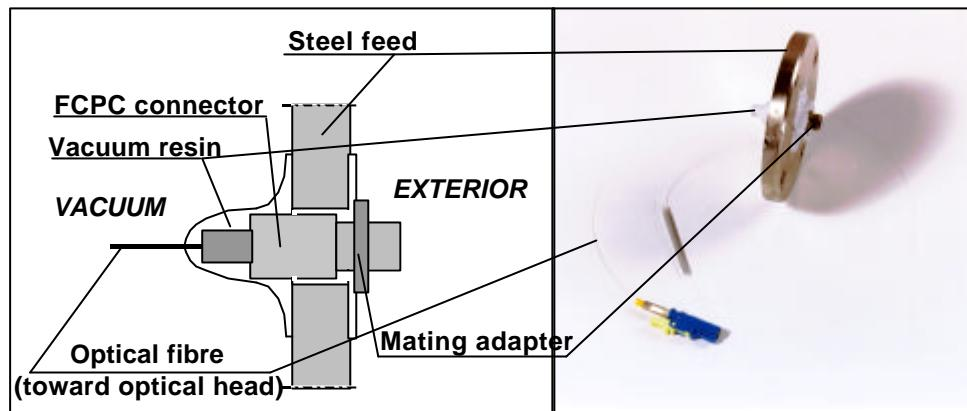
Figure 3: Schema and photo of feedthrough prototype
