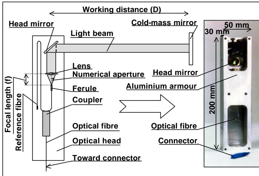
Figure 2: Schema, photo and principle of functioning of Displacement Sensor
