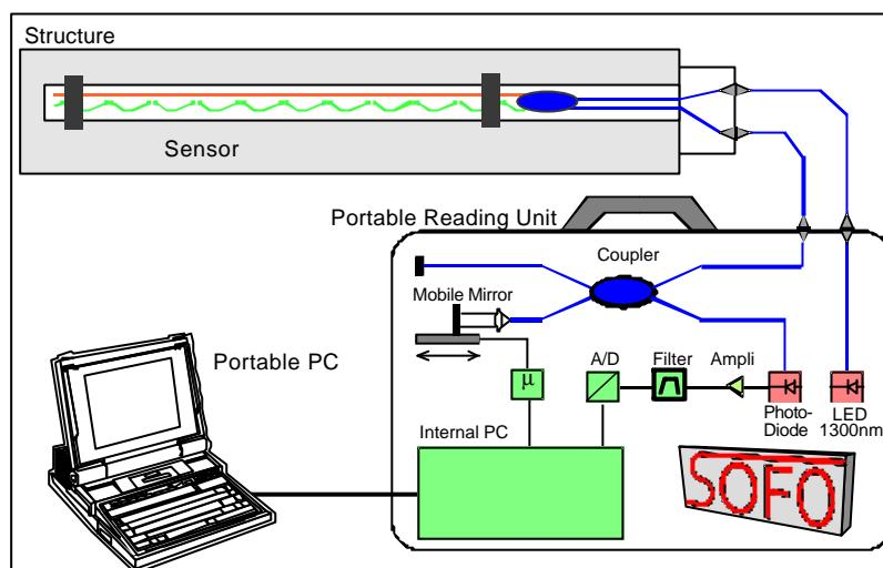
Figure 1: Set-up of the SOFO System
