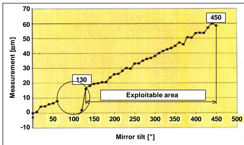
Figure 10: Vertical tilt measurements
