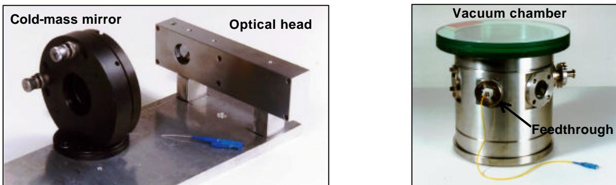
Figure 5: Optical head and cold-mass mirror placed in vacuum chamber, and chamber it-self with installed feedthrough
