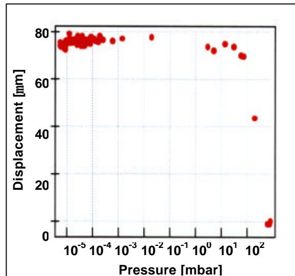
Figure 9: Displacement Sensor measurements with respect to pressure
