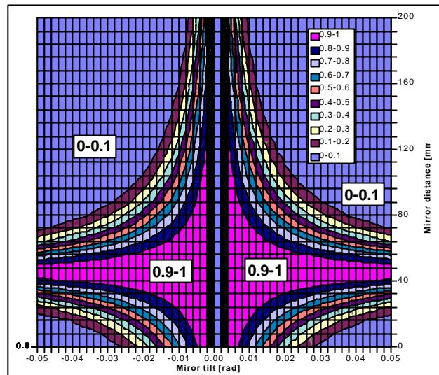
Figure 7: Theoretical back coupling efficiency of the sensor
