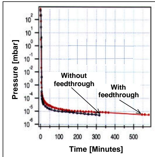
Figure 6: Vacuum tests of the prototype and the feedthrough
